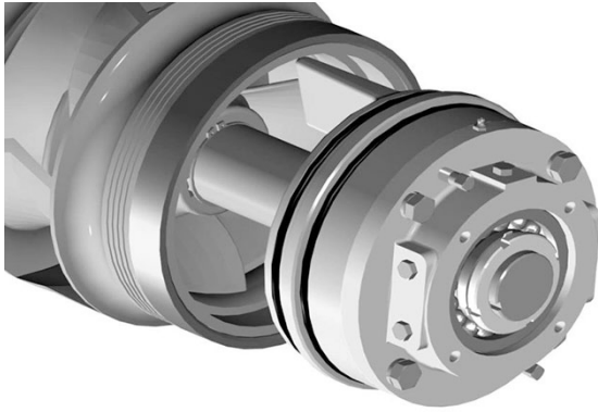
Figure 52: Lockwasher and locknut installed on outboard (opposite of coupling) end of rotating assembly
