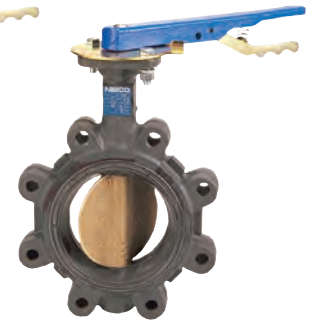
LD-2100 Lug Style Buna-N Liner and Aluminum Bronze Disc
